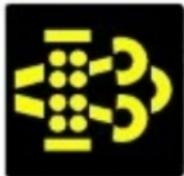
If the DPF light flashes yellow on the dash it means the vehicle needs to burn off the built-up diesel particles in the exhaust system. The vehicle must be stopped within 40km to allow the burn to take place.
